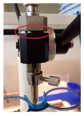
Adjusting of distance between rivet tip and frame.
