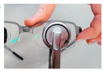
Depending on the blocking system it is advisable to remove the blockers before further working steps.
