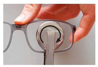
B Depending on the blocking system it is advisable to remove the blockers before further working steps
