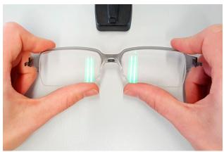
Fixing the hinge, positioning the temple parallel to the front, inserting the temple in the hinge until it clicks into place.
