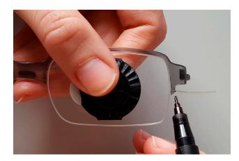
Moving the thread through the second hole and cut the overlay. The overlay has to be fitted tightly to the frame and lens shape.
