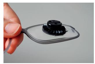
Lifting the lower frame carefully with little force over the edge of the lens.
