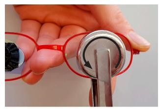
Fixing the frame at the bridge and the hinge the other way around to turn the lenses clockwise.
