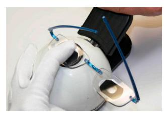
Press pad onto bolt of the bridge with mounting tool.
