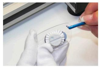
Make sure bridge and hinges fit closely to outside of lens.
