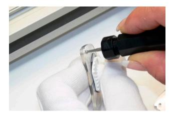
Insert bridge and hinges into long holes and press them on firmly.
