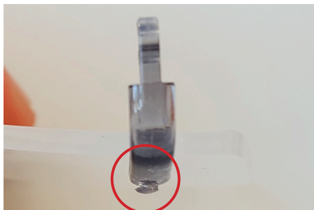
Rivet pin tilts sideways and is too big
