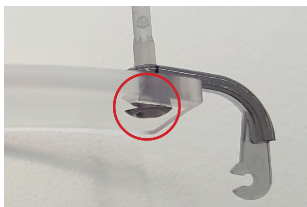
Rivet pin at an angle to lens surface
