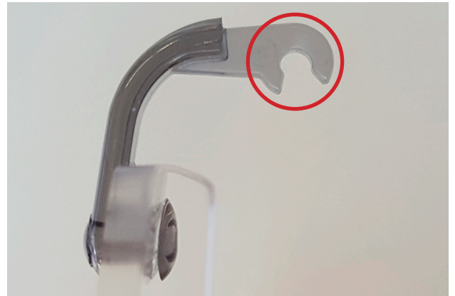
Hinge is widened (incorrect handling)
