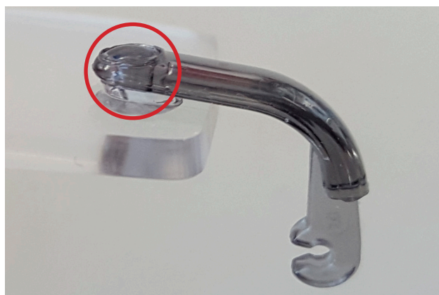
Rivet pin with edge (too much pressure or too much time – part has to be replaced)
